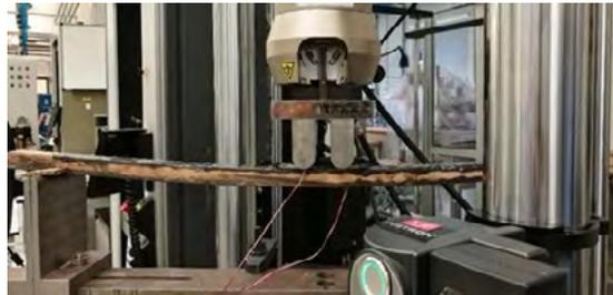
**Figure 3.** Experimental setup for 4-point flexural test with sandwich beam.
